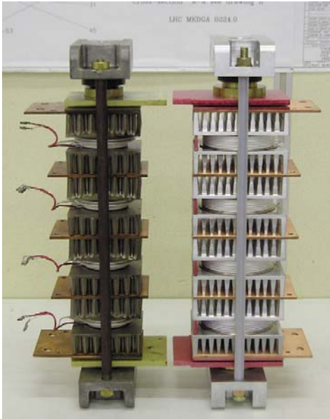
Figure 15, RCT and IGBT stacks
